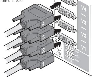
Note: On the rear panel of the unit, connectors belonging to the same channel are stacked vertically. The connectors at each horizontal level (V1 to V4) will be switched through to the user console DVI-I connector which is at the same level:
