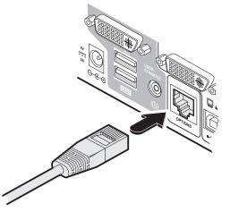
2 Connect the other end of the cable to a vacant serial port on the computer or to the output of the switching device.
