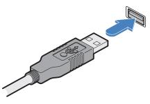
Connect the four USB cables to vacant USB ports on each computer
