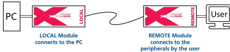
Hence, the LOCAL module connects directly to the system, while the REMOTE is at the other end of the twisted pair cable(s) and attaches to the video monitor, USB peripherals and sound equipment.
